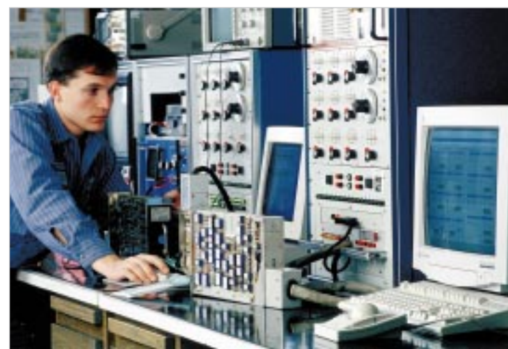
The new DATE-1b ATE test set in Duncan Aviation's Avionics Shop fully automates the testing procedures of certain autopilots and flight directors. Here, the set tests a Collins 562A-5M flight computer while Avionics Specialist Aaron Spulak works on a Sperry FZ500.
