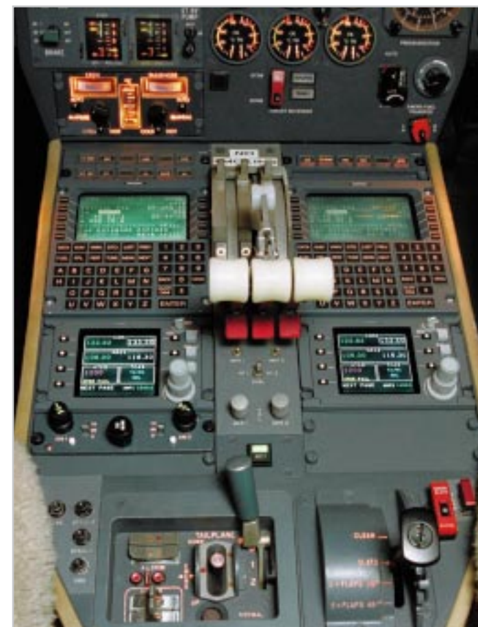
Duncan Aviation recently installed Collins' ProLine 4 retrofit package in this Falcon 50 aircraft to help ready it for service in the 21st Century. This package includes a fully digital autopilot with RVSM-compatible Air Data Computers, an updated instrument panel with large 7 1/4-inch EFIS displays, state-of-the-art Navigational and Communication Transceivers with compact Radio Tuning Units that yield high reliability and reduced weight, the Collins Doppler Radar and the capability to meet present and future FANS and MNPS requirements.
