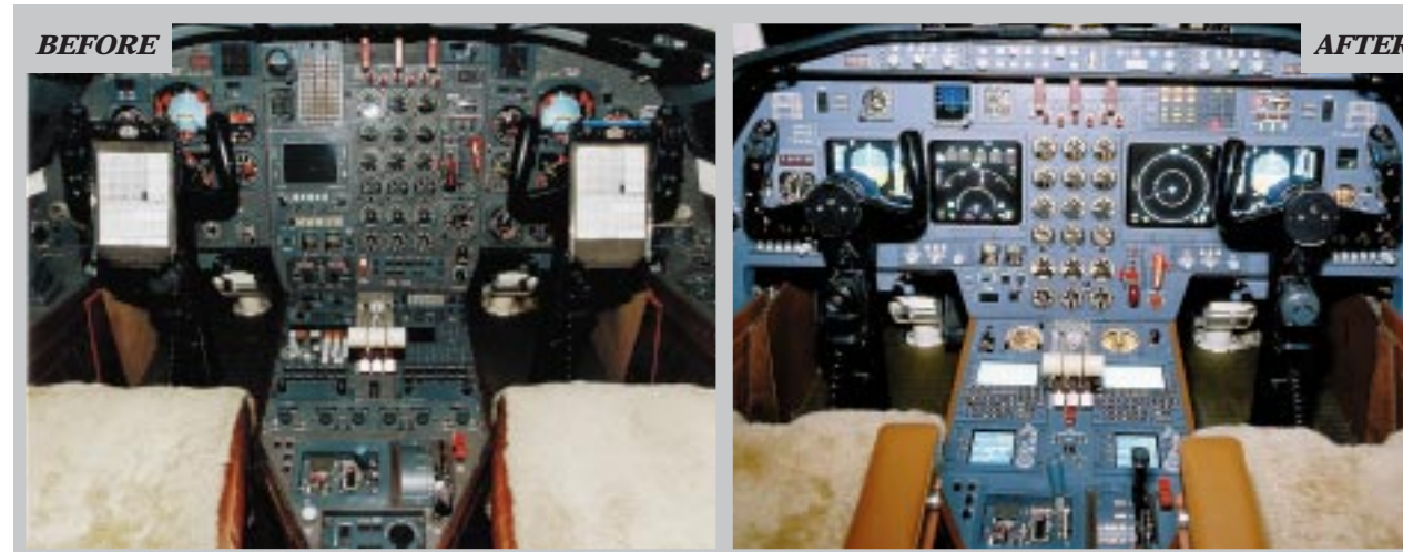
Duncan Aviation recently installed Collins' ProLine 4 retrofit package in this Falcon 50 aircraft to help ready it for service in the 21st Century. This package includes a fully digital autopilot with RVSM-compatible Air Data Computers, an updated instrument panel with large 7 1/4-inch EFIS displays, state-of-the-art Navigational and Communication Transceivers with compact Radio Tuning Units that yield high reliability and reduced weight, the Collins Doppler Radar and the capability to meet present and future FANS and MNPS requirements.
