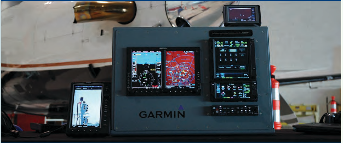
Garmin GTN-750 and GTN-650 touch-screen fully integrated GPS/NAV/COMM systems that were installed in a Pilatus PC-12/45 aircraft by Duncan Aviation-Denver.
