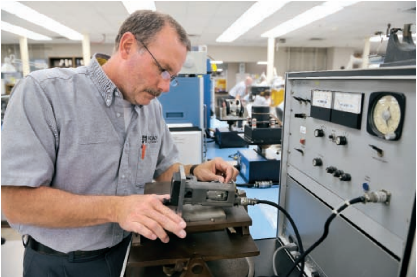
Jerry Bremer, gyro team leader for Duncan Aviation, utilizes his 30 years of gyro experience to calibrate a Sfena 803 horizon gyro.
