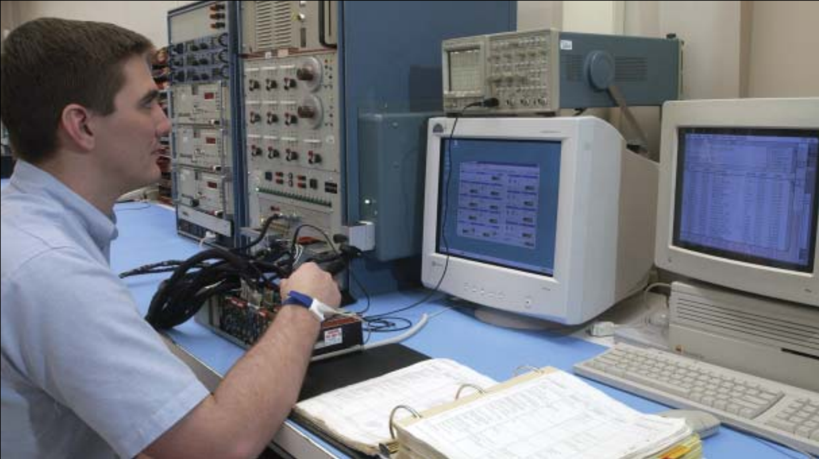
Brent Gillette, Duncan Aviation Autopilot Tech III, overhauls an autopilot unit.
