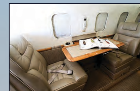
New seats, carpet, headliner and sidewalls, including LED lighting and lavatory refurbishment.
