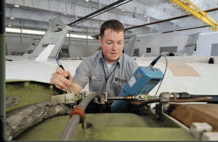
Casey Fix conducting an Eddy Current inspection on a Challenger's "Nose Cowl Actuator Support Fittings - Forward Attachment Lugs."
