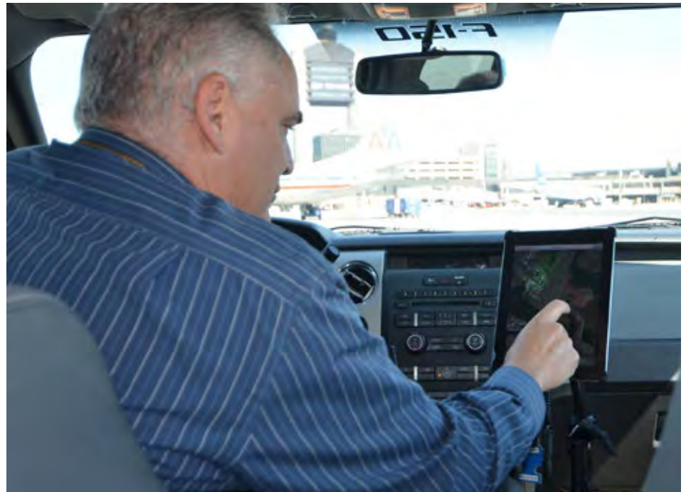
Ground vehicles equipped with ADS-B enhance safety on the airport surface as part of a demonstration project at Boston.
