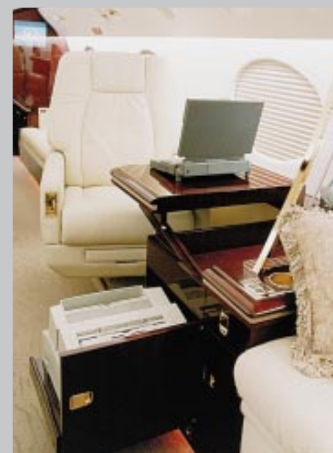
A workstation was designed for the left-hand side of the aircraft that includes a pentium notebook, a laser printer/fax machine, office supply storage and an adjustable-height worksurface. (Left)
