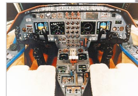
The Collins Pro Line IV retrofit will upgrade a Falcon 50's avionics to meet needs for years to come.
