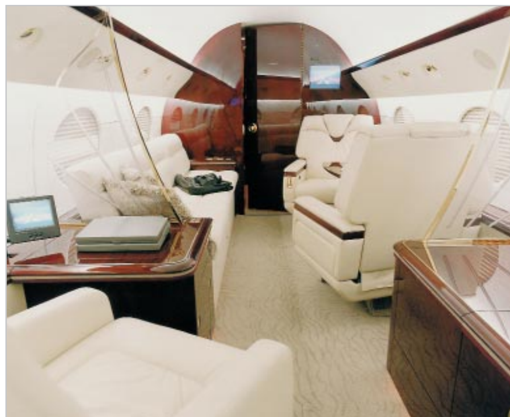
New GIV-style seats were installed in this GII completion. The forward two were styled for "executive seating" and a berthable divan was installed for sleeping. Two double clubs were installed in the aft cabin.
