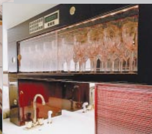
New galley towers were designed and installed to display the customer's wine and champagne glasses. The galley base was radiused to present a clean, updated look and the countertops were custom-finished with a white carrera faux marble. (Below)
