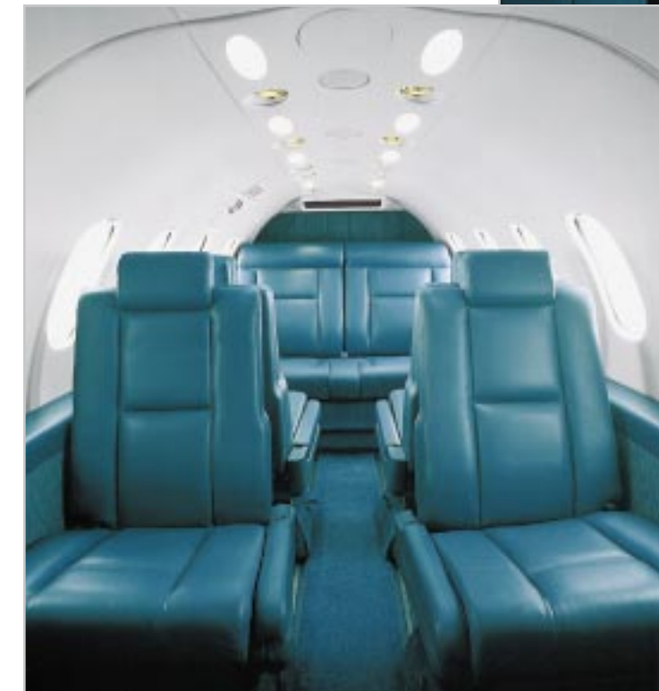
This Learjet 31 recompletion included a fold-down work surface for beverage and food service. The cabinetry also sported newly designed hardware (latches and hinges) created for Duncan Aviation by Sealth Aero Marine.
