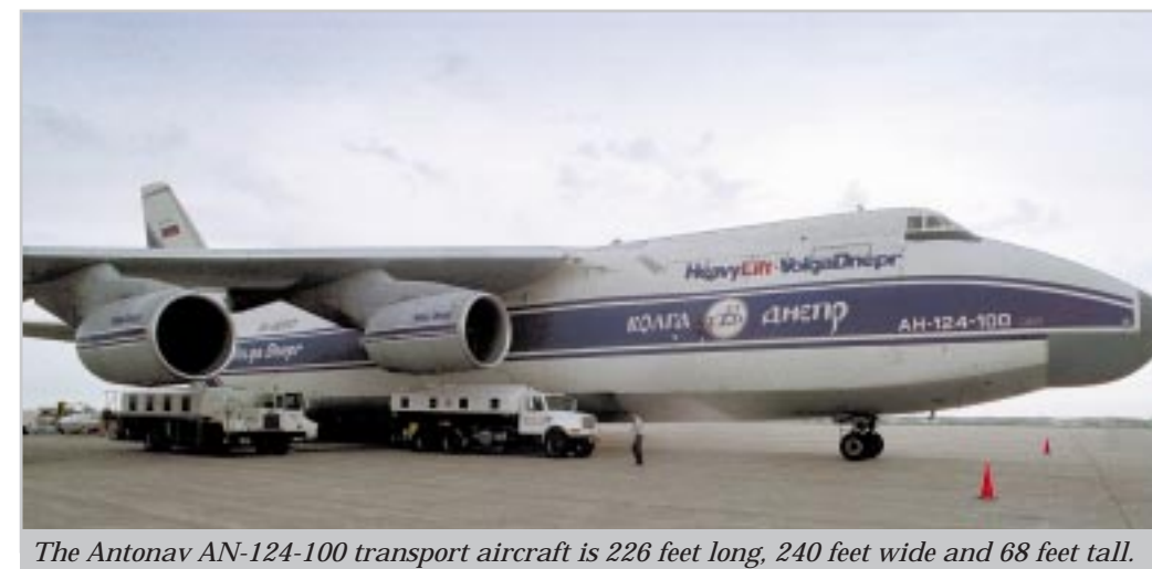
The Antonov AN-124-100 transport aircraft is 226 feet long, 240 feet wide and 68 feet tall.
