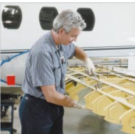
Structural repair mechanic Dave Cox repairs structural damage to a Citation 501 incurred in a ground incident.
