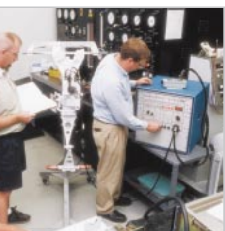
Prop/Accessory Team Leader Vince Cruickshank and R & D Technician Chris Hoagg adjust and test a Challenger's nose gear steering system.
