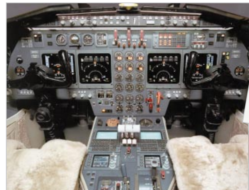
The ProLine 4 avionics retrofit package updates the entire Falcon 50 cockpit. This was the second ProLine system installed by Duncan Aviation. (The first Duncan installation was delivered in October 1997 in Lincoln.)
