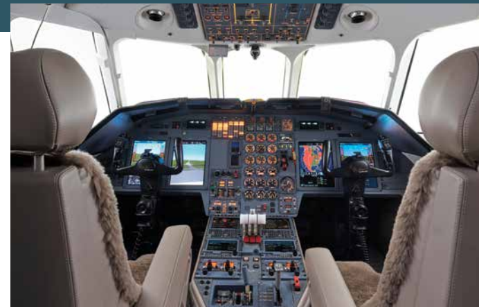
Duncan Aviation installed the Universal Avionics InSight Flight Display System in a Falcon 900B, replacing obsolete CRT equipment with bright, crisp displays that provide cutting-edge, 3D graphics for the SVS (Synthetic Vision System), weather, terrain, and traffic systems.
