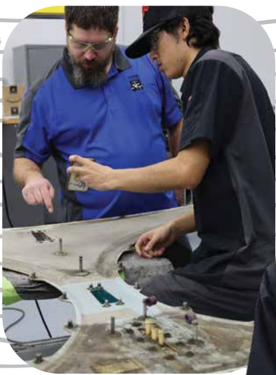
Inspecting Composites For Contamination
