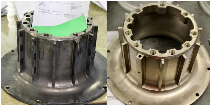
Before and after the Nickel plating restoration
