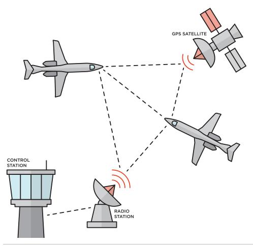
these signals and rebroadcast them for other aircraft to see, effectively merging the 1090 and 978 MHz systems. The rebroadcast traffic service is referred to as Traffic Information Services-Broadcast (TIS-B). Other aircraft can directly receive these signals if both aircraft are equipped to do so. ATC uses the aircraftbased information to tighten the lateral separation at altitude and tighten the lateral and vertical separation when the aircraft is ascending or descending through airspace.
