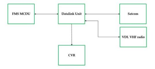
**Datalink.** The heart of any FANS installation is the datalink unit. Each equipment provider has a datalink unit that has FANS or FANS/ATN capability. The datalink will interface with the FMS (Flight Management System) to provide a connection between the crew in the cockpit and ATC. The crew will log on to the applicable network to establish the connection between the aircraft and ATC.
