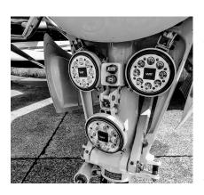
**Exterior Lighting**—There are a number of exterior aircraft lighting systems. Required lighting includes navigation (position) lights and anti-collision strobe or beacon lights. Other common exterior lighting includes landing lights, taxi lights, logo lights, and pylon (for baggage load area). In addition to LEDs, HID (High Intensity Discharge) lights are another option available for landing and taxi lights.
