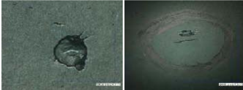
Figure 8 – Pinhole caused by static (left) or FOD (right)
