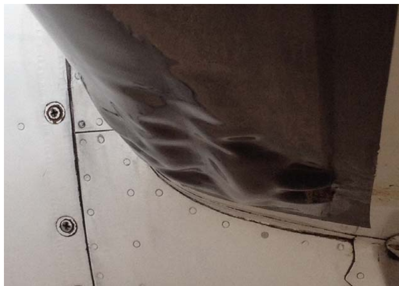
Figure 11 – Fuel Contamination Example
