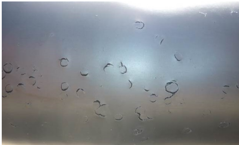
Figure 10 – Cold Impact Damage Example
