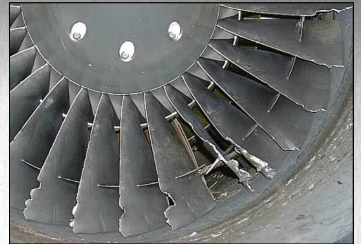
The damage to the TFE731 engine above was caused by a bird strike. Duncan Aviation's technicians found damage to the fan blades, nose cowl leading edge, fan stator, and compressor impeller... just to name a few. Depending on the strike, one bird can cause more than half-a-million dollars in damages.
