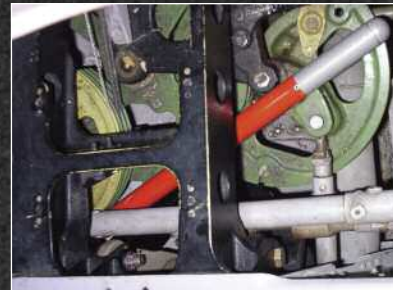
Duncan Aviation's technicians found this red Auxiliary Gear Handle (which belongs to the aircraft) sitting on top of the flight control pulleys.
